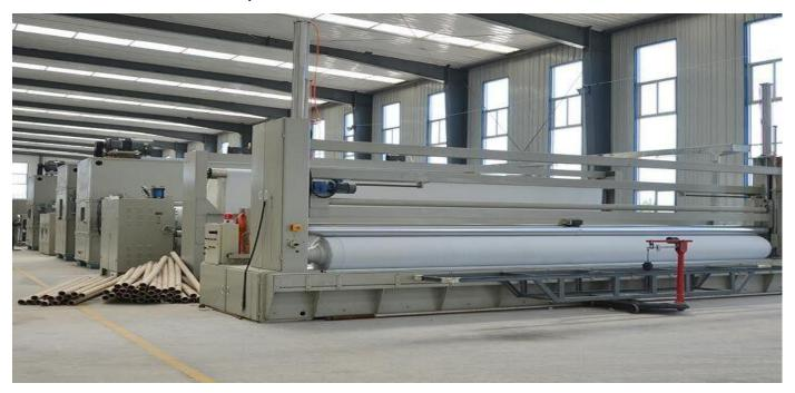
The Third Production Line: Staple Fiber Needle-Punched Nonwoven Geotextile
